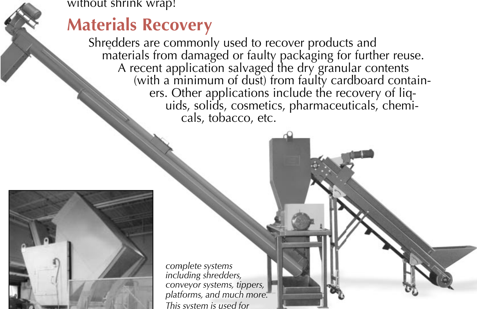
This system was designed for a major oil company to recover oil product from damaged 1-quart plastic bottles. The system includes a MS1714 Shredder, a flat belt infeed conveyor, and screw discharge conveyor with liquid/solid separation capability.
